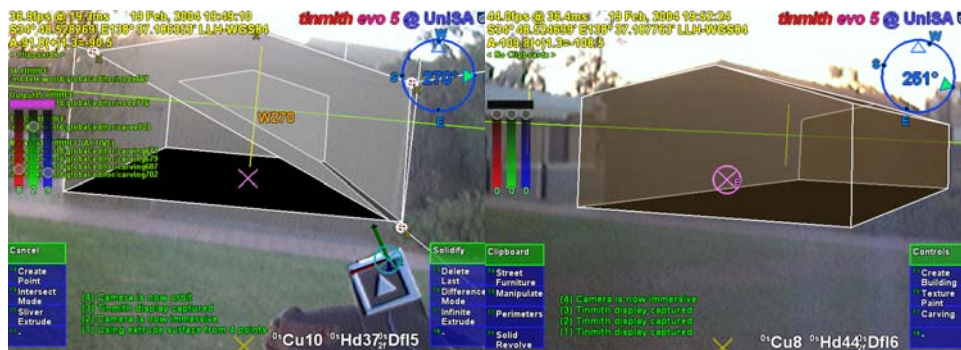
Figure 4. AR views of an infinite planes building with sloped roof being interactively carved
