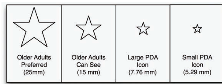
Figure 1. Example of icon sizes older adults can view (preferred size and smallest viewable size) on a PDA
